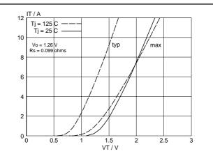
Fig.10. Typical and maximum on-state characteristic.
