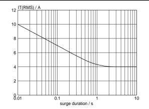
Fig.5. Maximum permissible repetitive rms on-state current  $I_{T(RMS)}$ , versus surge duration, for sinusoidal currents, f = 50 Hz;  $T_{mb} \le 113 ^{\circ}\text{C}$ .
