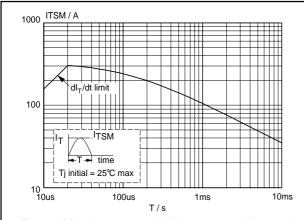
Fig.2. Maximum permissible non-repetitive peak on-state current  $I_{TSM}$ , versus pulse width  $t_p$ , for sinusoidal currents,  $t_p \le 10$ ms.
