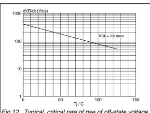
Fig.12. Typical, critical rate of rise of off-state voltage, dV<sub>D</sub>/dt versus junction temperature T<sub>i</sub>.
